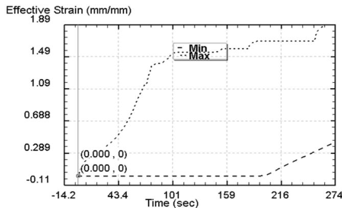
Figure 9: Relationship of effective strain and time.
