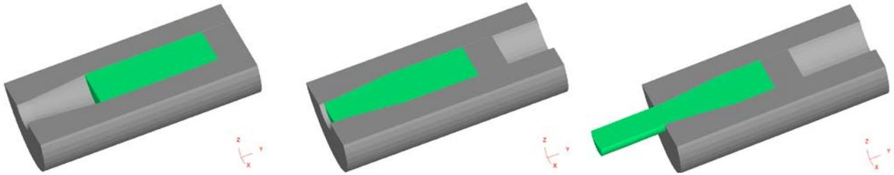
Figure 4: Simulation analysis of an extrusion die process; a) before extrusion; b) middle extrusion; and c) after extrusion.
