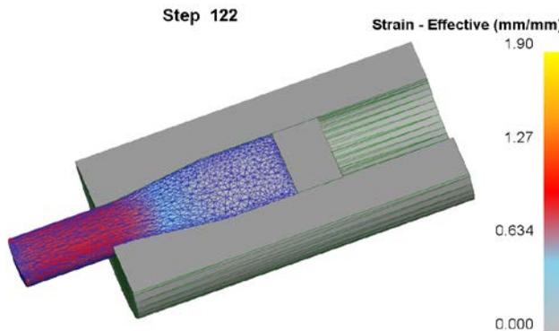
Figure 7: Strain effective of billets extruded.
