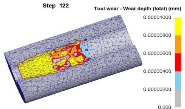
Figure 8: Simulation analysis of tool wear.
