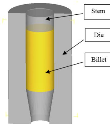
Figure 2: Extrusion die designed.
