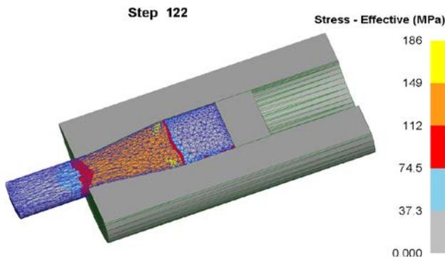
Figure 5: Effective stress of simulation analysis.
